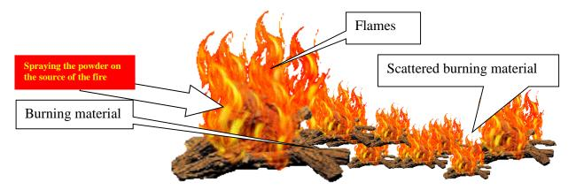
Figure 5 The fire spreads when the powder is sprayed on the source of the fire
