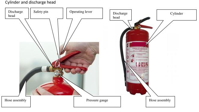
Figure 1 The parts of a powder extinguisher
